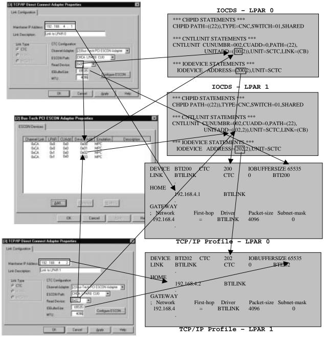
Figure 5-23. Multiple TCP/IP Direct Connect ESCON Configuration
